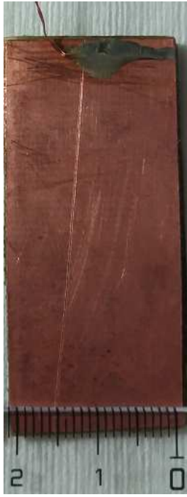
FIG. 3. Textolite plate with Copper foils on both sides, and with an electrode wire attached at the top.
